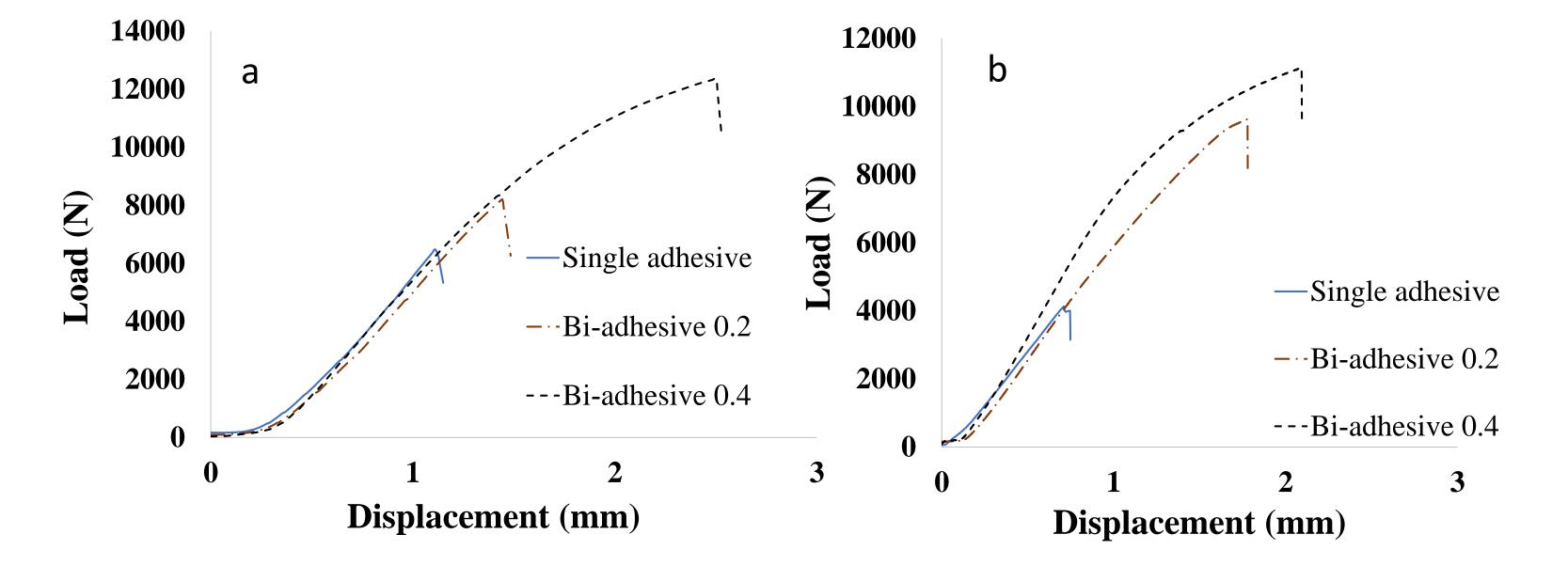
Figure 4 – (a) Typical load displacement behavior of specimens in static conditions; (b) Typical load-displacement behavior of specimens in dynamic conditions
