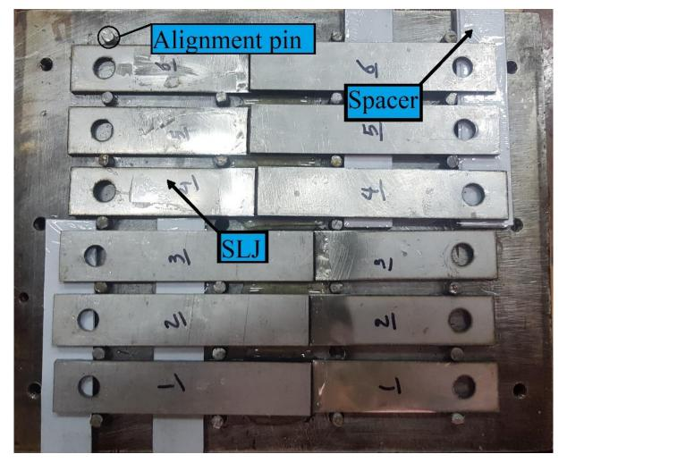
Figure 1 - Mold used for the manufacturing of SLJs
