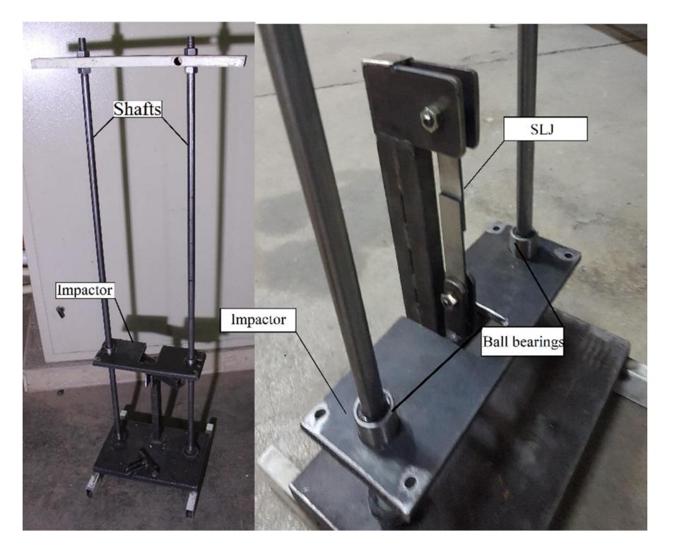
Figure 3 – Inhouse designed drop weight impact test machine
